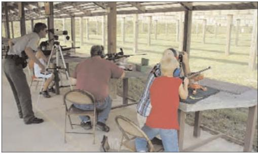
Covered shooting lines and and baffles can prevent bullets from being fired in an unsafe direction. Downrange, a berm with bullet catchers stop all bullets.
